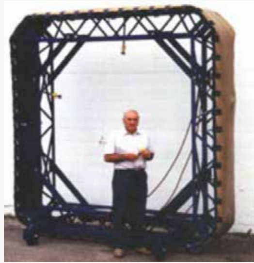
Square mainline packer for Box Culverts
