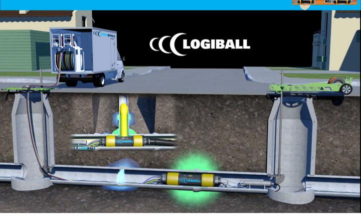
Chemical grouting was originally developped in 1955 as a technique for soil stabilization. Since then, it has been used to stop groundwater infiltration in sewers, manholes, chambers, subways, mines, tunnels and many more underground structures all over the world. Recent studies, combined with over 60 years of experience, show that the original trenchless technology remains the first line of defense and the best long term ROI against groundwater infiltration in structurally sound sewers.
